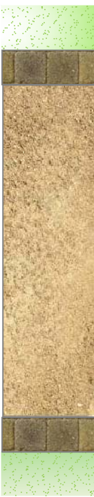
Footpath - Bound gravel & sett kerb - Plan
